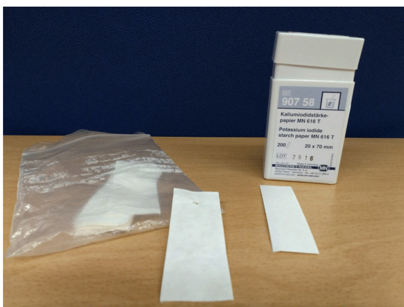
Figure 7: Comparison between the measurement paper strip manufactured following the procedure exposed here (left) with a commercially supplied one (right).
