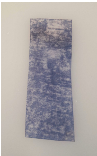
Figure 6: Strip collected, from which to take the measurement, after being exposed for 24 hours outdoors and immersed in distilled water.
