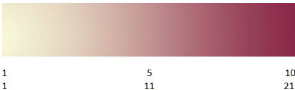
Figure 3: Ozone strip measurement color scale. Values from 1 to 10 (top row) correspond to the Schönbein scale. Values of 1 to 21 (lower row) correspond to the Berigny scale.
